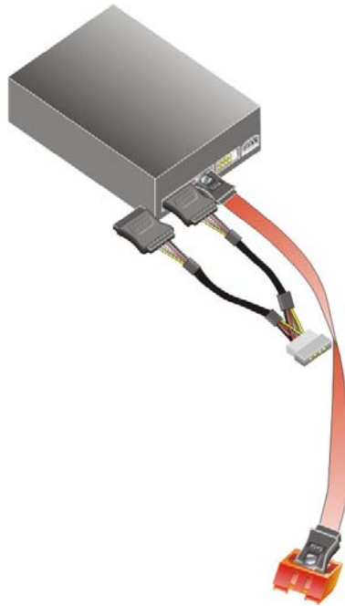
Figure 4-14: SATA Power Drive Connection
