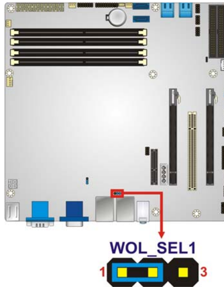
Figure 4-12: Wake-on LAN Connector Pinout Locations
