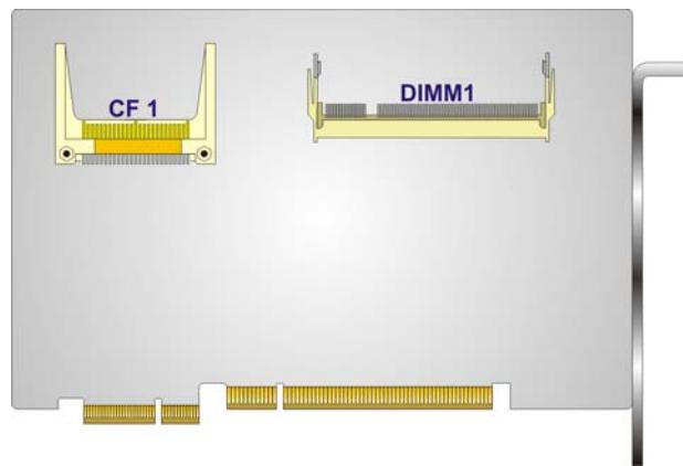
Figure 3-2: Connector and Jumper Locations [Solder Side]
