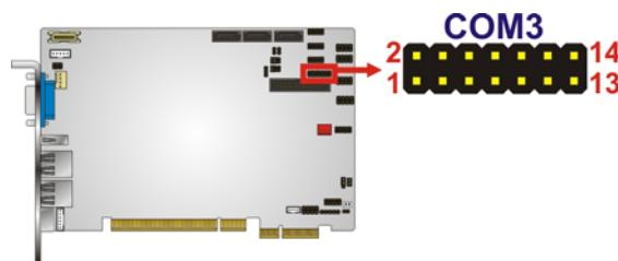
**Figure 3-16: Serial Port Connector Location**
