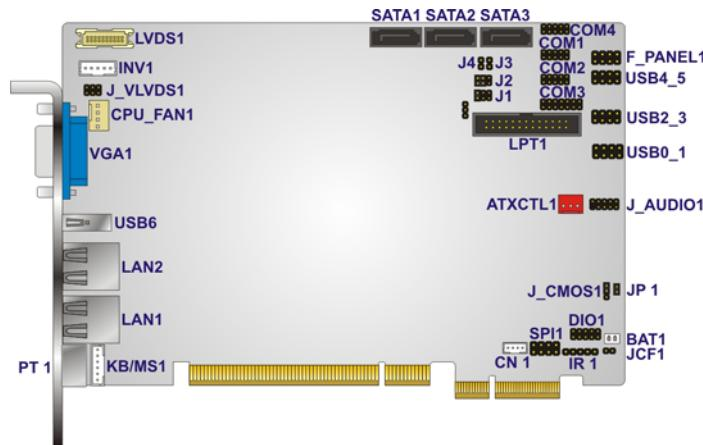
Figure 3-1: Connector and Jumper Locations [Front Side]
