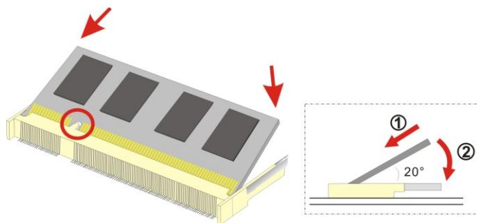
**Figure 4-1: SO-DIMM Installation**
