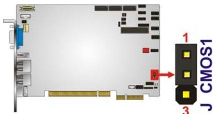
**Figure 4-6: Clear CMOS Jumper**
