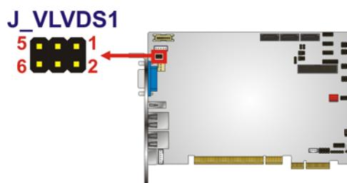
**Figure 4-7: LVDS Voltage Selection Jumper Pinout Locations**
