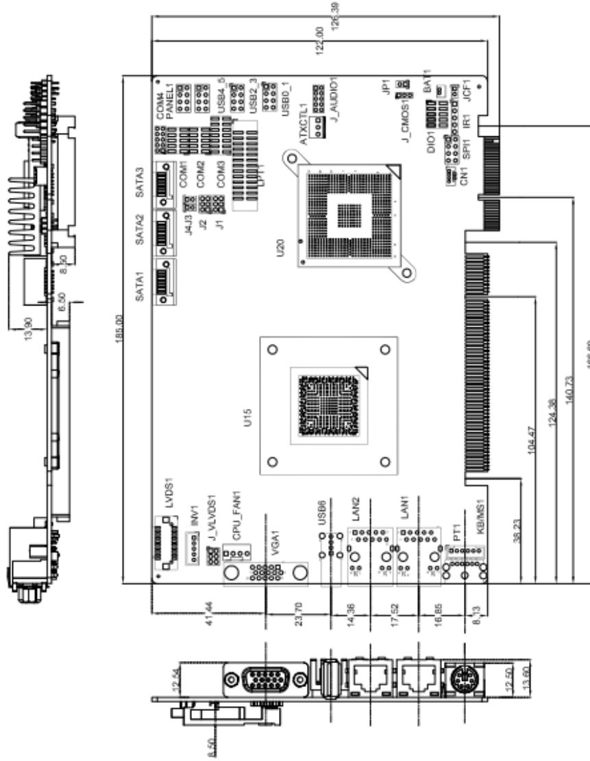
Figure 1-3: PICOE-PV-D4251/N4551/D5251 Dimensions (mm)
