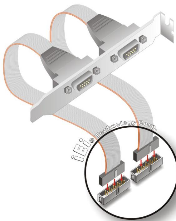
**Figure 4-17: Dual RS-232 Cable Installation**
