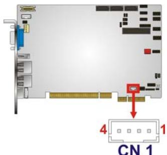
**Figure 3-17: SMBus Connector Locations**
