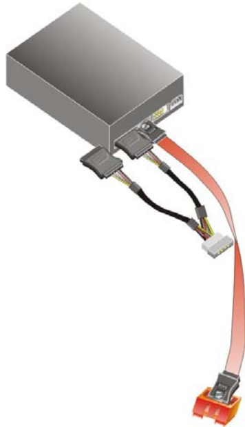
Figure 4-10: SATA Power Drive Connection
