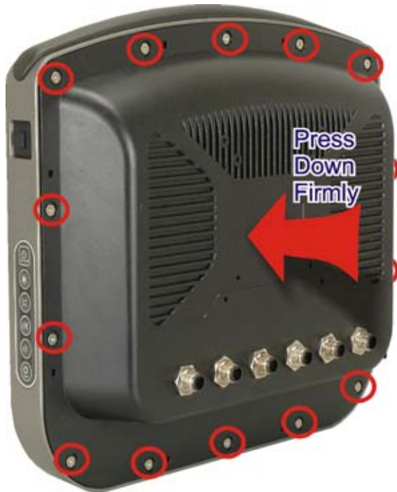
Figure 6-5: Rear Cover Screws
