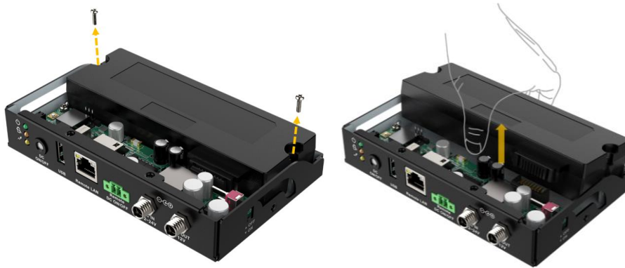
Figure 3-3: Battery Pack Installation
