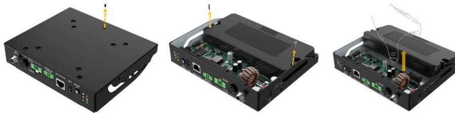
Figure 3-2: Battery Pack Installation
