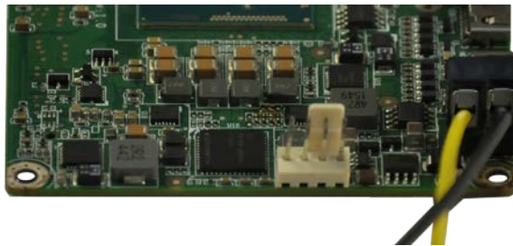
Figure 4-6: Power Cables Connection
