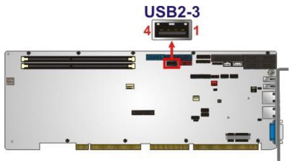
Figure 3-30: USB 2.0 Connector (Type A) Pinout Location
