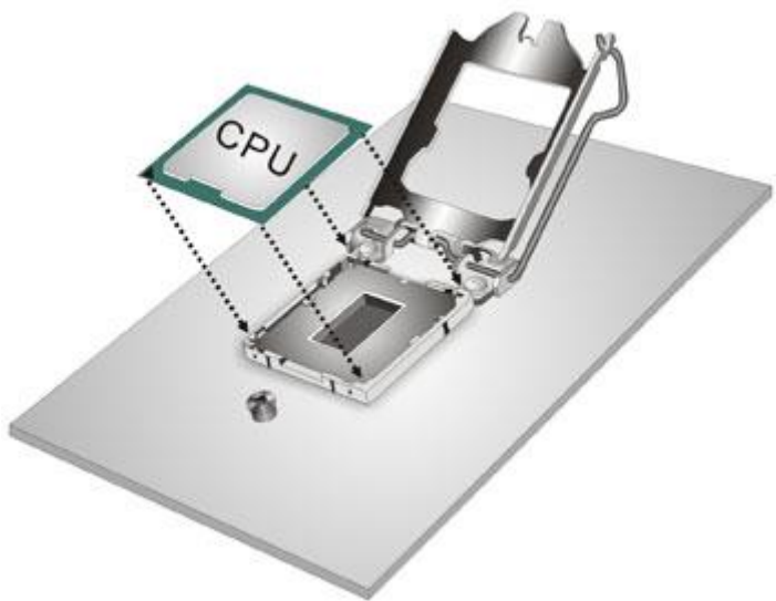
Figure 4-3: Insert the Socket LGA1150 CPU
