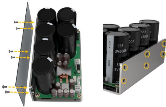
Figure 3-6: Secure the RHEA-I660A – from Side
