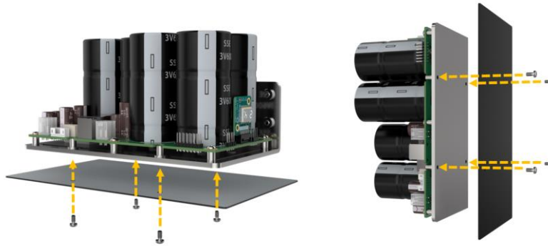
Figure 3-3: Secure the RHEA-I660A – from Bottom
