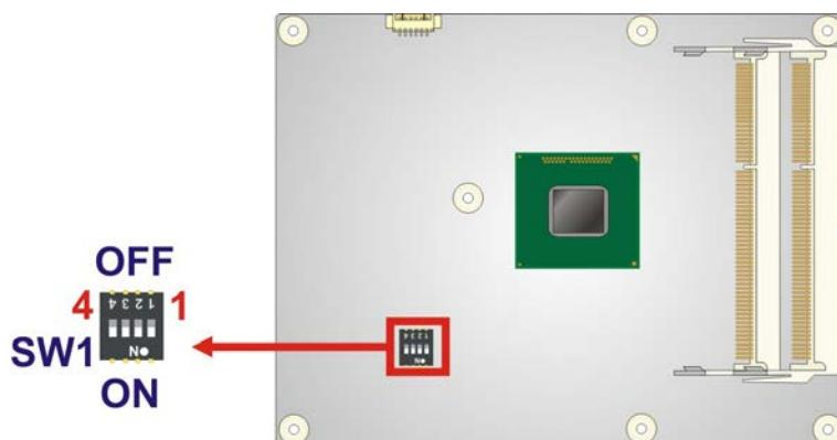
Figure 4-2: LVDS Panel Type Selection Switch Location
