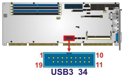
**Figure 3-30: USB 3.2 Gen 1 Connector Location**
