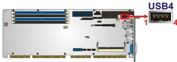
**Figure 3-29: USB 2.0 Connector (Type A) Pinout Location**
