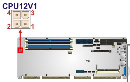
**Figure 3-2: +12V ATX Power Connector Pinout Location**
