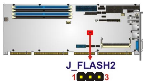
**Figure 4-17: Flash Descriptor Security Override Jumper Location**
