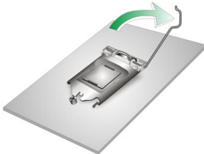
**Figure 4-1: Disengage the CPU Socket Load Lever**
