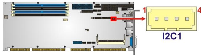
**Figure 3-13: I<sup>2</sup>C Connector Location**
