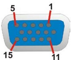
**Figure 3-33: VGA Connector**
