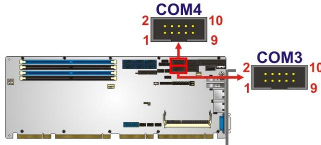
**Figure 3-22: RS-232/422/485 Serial Port Connector Locations**
