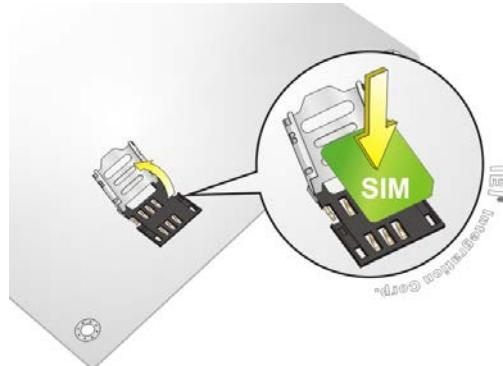
Figure 4-13: SIM Card Installation
