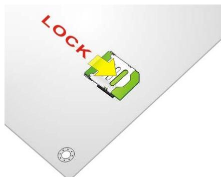
Figure 4-14: Lock SIM Card Slot Cover
