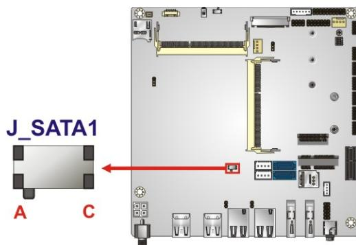
**Figure 4-20: M.2 and SATA2 Select Switch Location**
