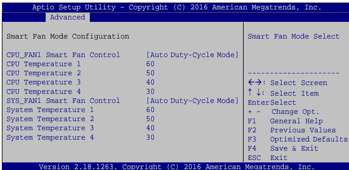
**BIOS Menu 8: Smart Fan Mode Configuration****→ CPU\_FAN1/SYS\_FAN1 Smart Fan Control [Auto Duty-Cycle Mode]**
