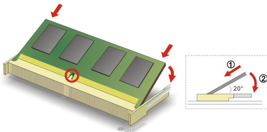
**Figure 4-1: SO-DIMM Installation**
