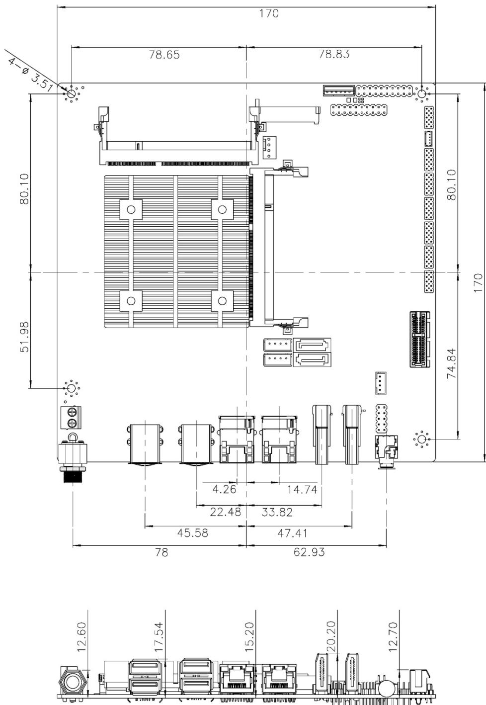
Figure 1-4: Dimensions (mm)
