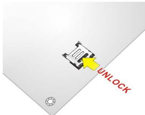
Figure 4-12: Unlock SIM Card Slot Cover
