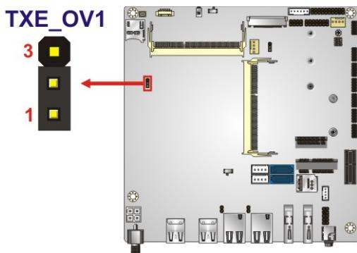
**Figure 4-19: Flash Descriptor Security Override Jumper Location**
