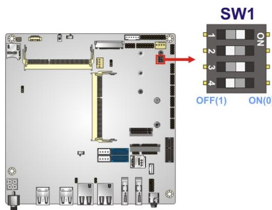
**Figure 4-17: COM1 and COM2 Function Select Switch Location**
