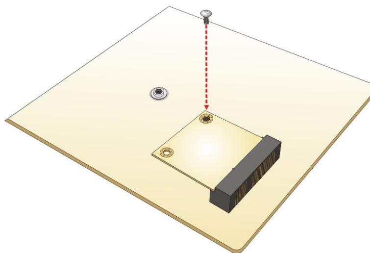
Figure 4-11: Securing the Half-size PCIe Mini Card
