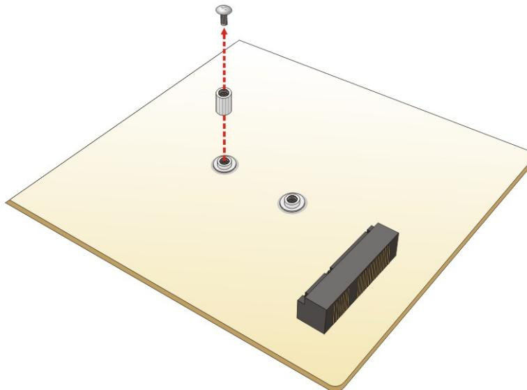
**Figure 4-8: Removing Retention Screw and Standoff**
