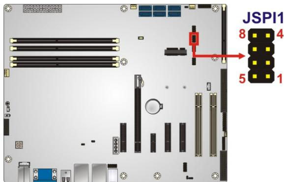
**Figure 3-30: SPI Flash Connector Location**
