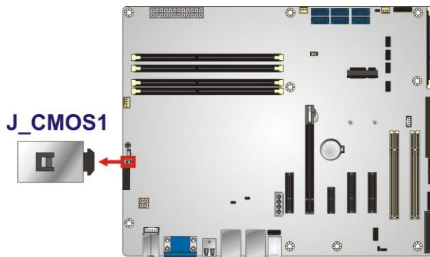
Figure 4-12: Clear CMOS Button Location
