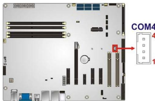
**Figure 3-28: RS-422/485 Connector Location**
