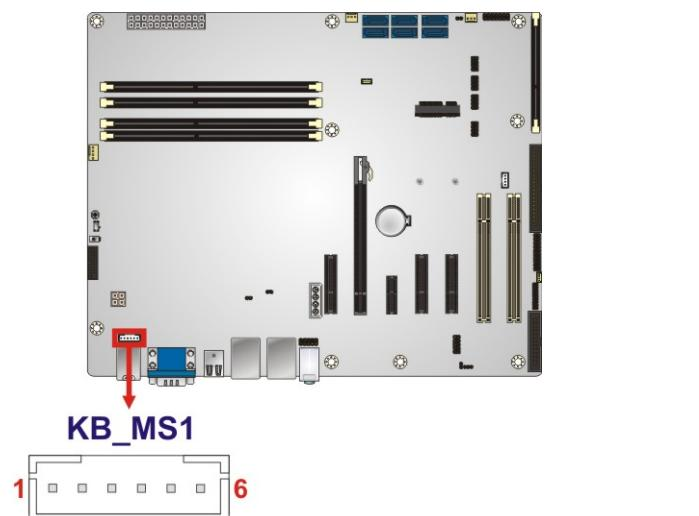
**Figure 3-17: Keyboard and Mouse Connector Location**
