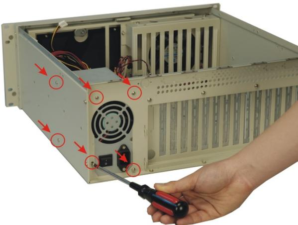
Figure 6: Insert PSU Retention Screws
