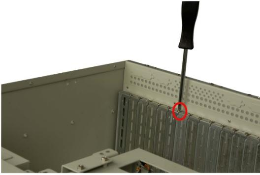
**Figure 8: Remove the Slot Cover Retention Screw**
