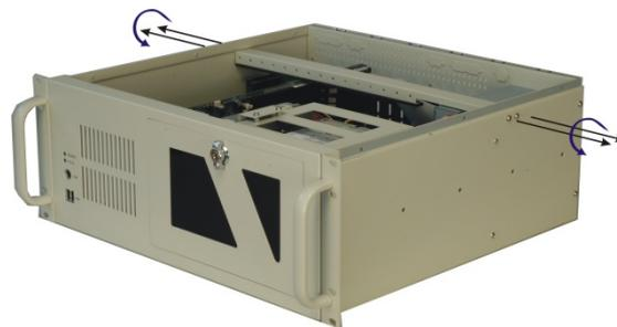
Figure 5: Remove the Hold-Down Clamp
