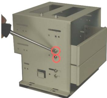
**Figure 12: Remove the Front Metal Cover Retention Screws**
