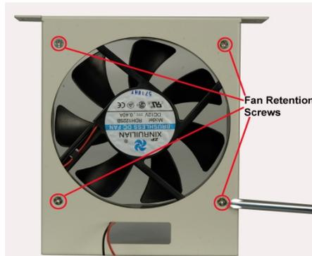
**Figure 18: Remove the Fan Retention Screws**
