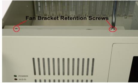
**Figure 17: Remove the Fan Bracket**
