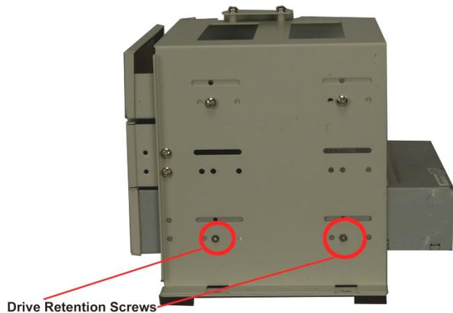
**Figure 14: Install 5.25" Optical Drive Retention Screws**
