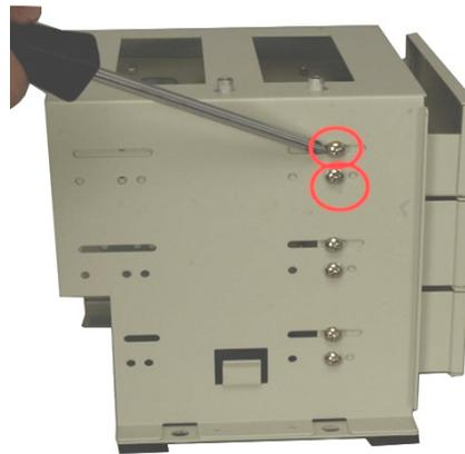
**Figure 13: Remove the 3.5" Drive Tray Retention Screws**
