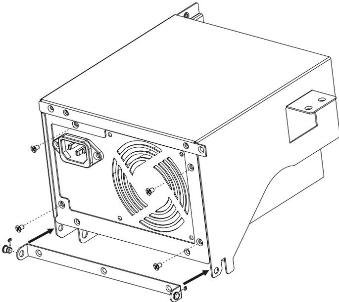
**Step 3: Secure the PSU bracket to the chassis.** Secure the PSU bracket to the chassis with the screws as figure shown below.
