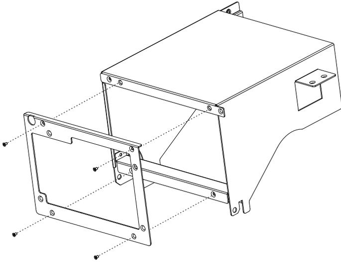
**Step 2: Install the PSU to the PSU bracket.** To install the PSU to the PSU bracket, secure the PSU with the screws as figure shown below. Make sure the power socket and the PSU fan face the rear of the chassis.
