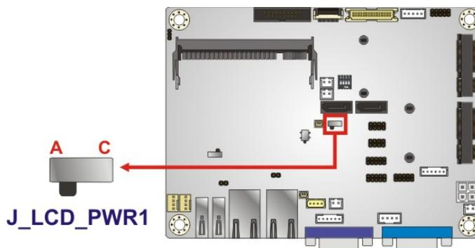
**Figure 4-12: LVDS Voltage Selection Jumper Location**
