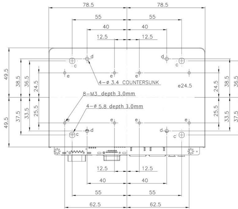
Figure 1-3: Dimensions (mm)
