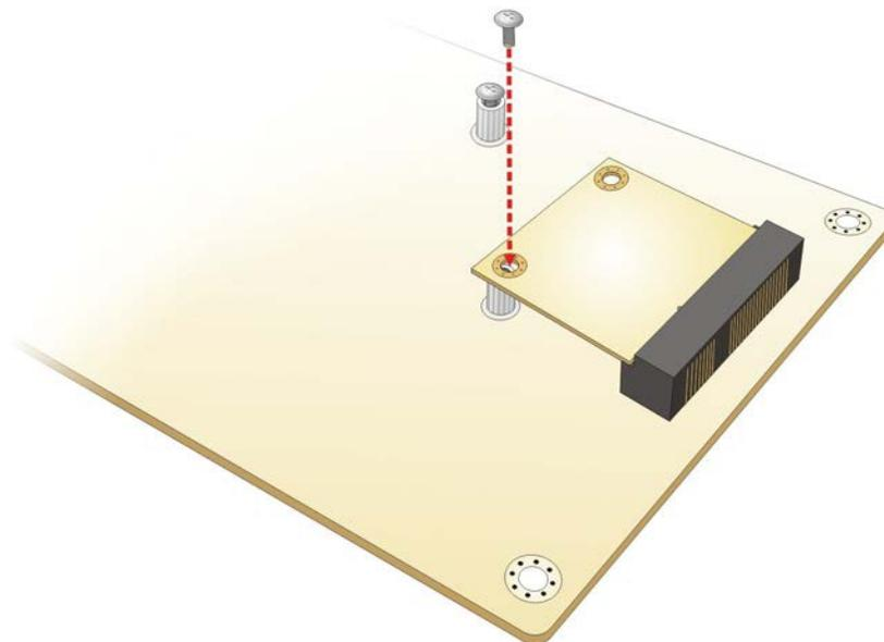
Figure 4-8: Securing the Half-size PCIe Mini Card
