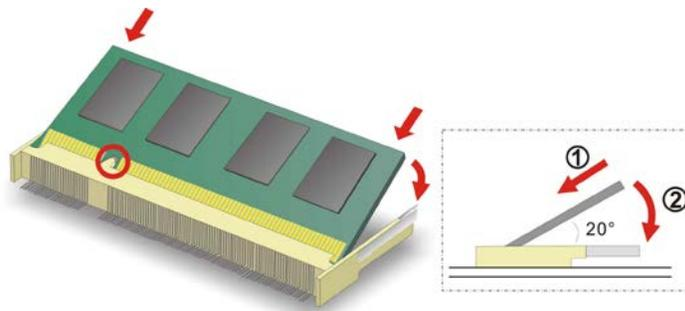
**Figure 4-1: SO-DIMM Installation**
