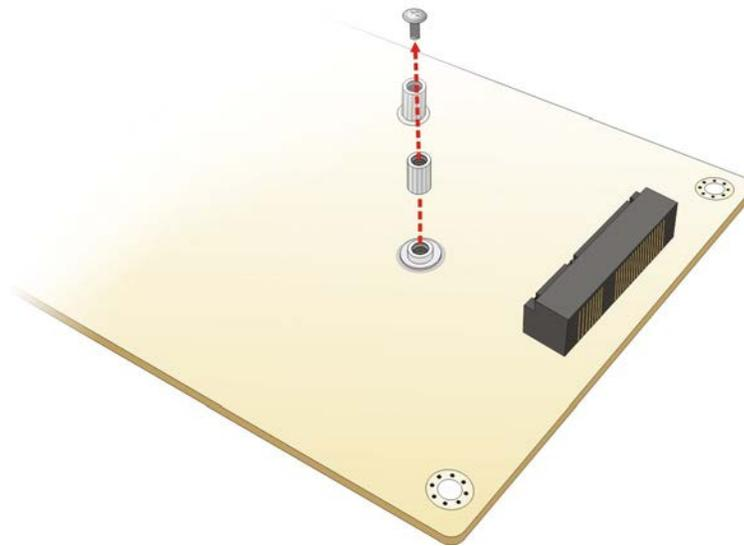
Figure 4-3: Removing the Retention Screw and Standoff
