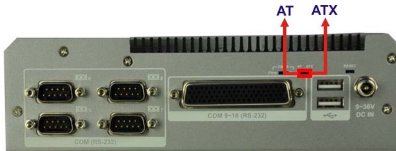
Figure 3-9: AT/ATX Switch Location
