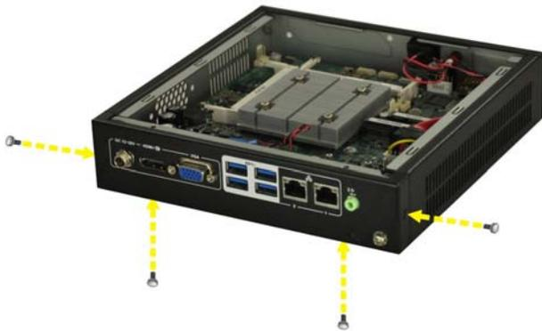
Figure 6: I/O Shielding Installation
