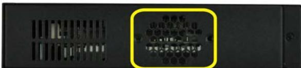
Figure 14: Vents for System Fan
