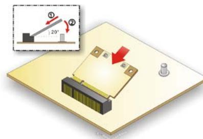
Figure 11: Inserting the WLAN Module
