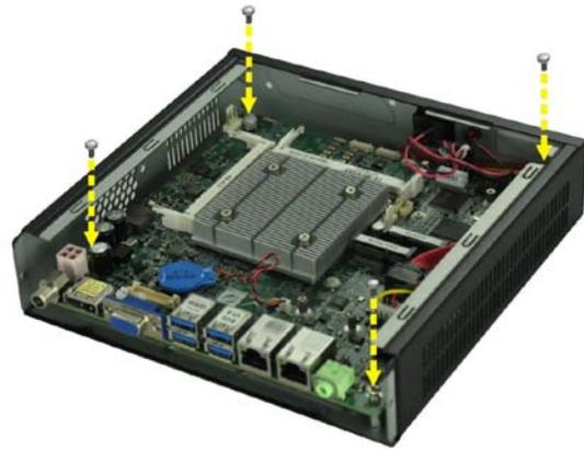
Figure 3: Motherboard Retention Screws
