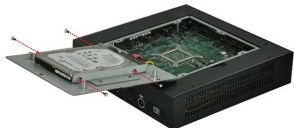
Figure 17: HDD Retention Screws
