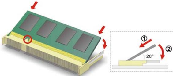
Figure 8: SO-DIMM Installation
