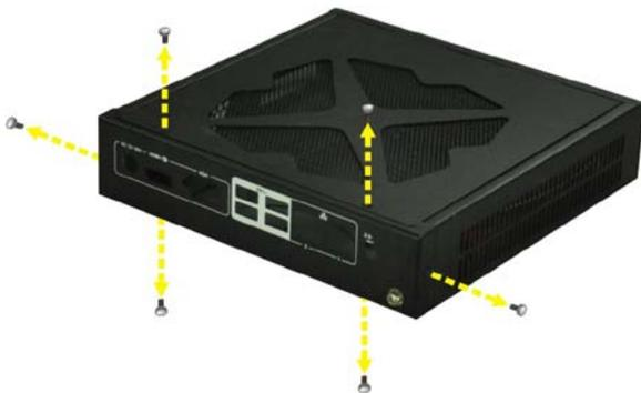
Figure 2: Remove the Top Cover and I/O Panel
