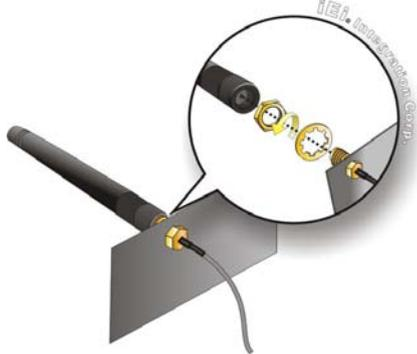
Figure 13: Securing SMA Connector and External Antenna
