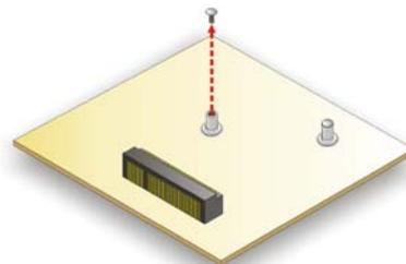
Figure 10: Removing the Retention Screw
