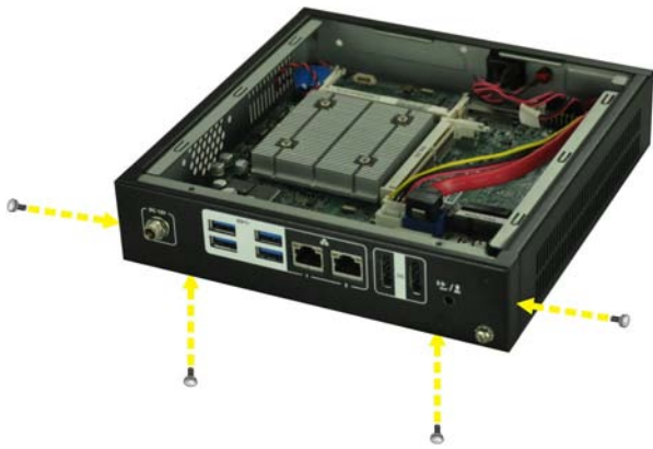
Figure 5: I/O Shielding Installation
