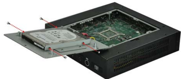
Figure 16: HDD Retention Screws
