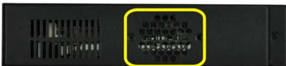
Figure 13: Vents for System Fan
