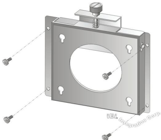
**Step 6:** Insert the four monitor mounting screws provided in the wall mount kit into the four screw holes on the rear panel of the medical panel PC and tighten until the screw shank is secured against the rear panel.
