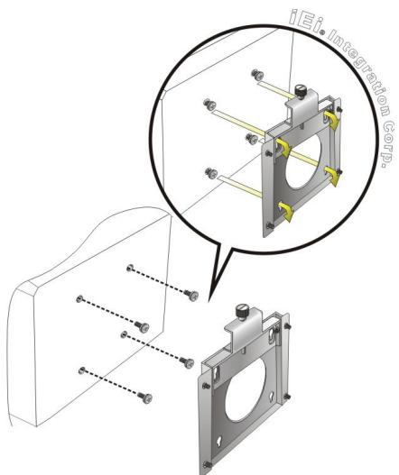
**Step 9:** Secure the panel PC by fastening the retention screw of the wall-mounting bracket.
