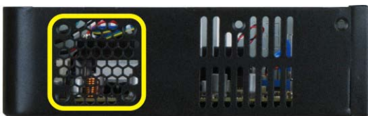
Figure 13: Vents for System Fan
