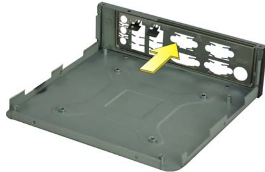
Figure 3: I/O Shielding Installation
