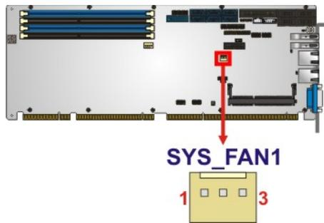
**Figure 3-10: System Fan Connector Location**
