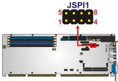
**Figure 3-23: SPI Flash Connector Location**
