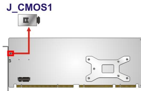
**Figure 4-8: Clear CMOS Button Location**
