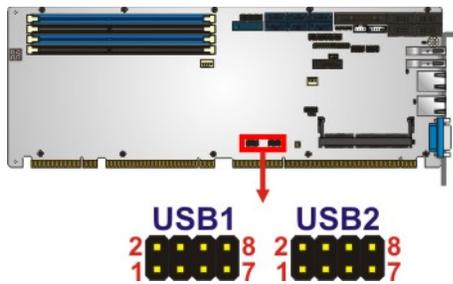
**Figure 3-26: USB 2.0 Connector Pinout Locations**
