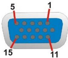
**Figure 3-30: VGA Connector**
