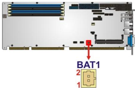
**Figure 3-4: Battery Connector Location**
