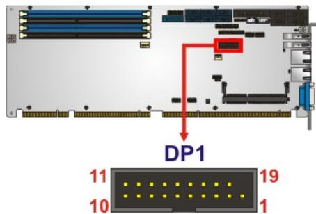
**Figure 3-12: Internal DisplayPort Connector Location**
