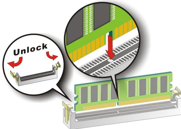
**Figure 4-6: DIMM Installation**
