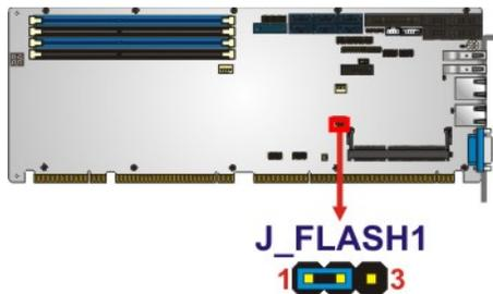
**Figure 4-9: Flash Descriptor Security Override Jumper Location**
