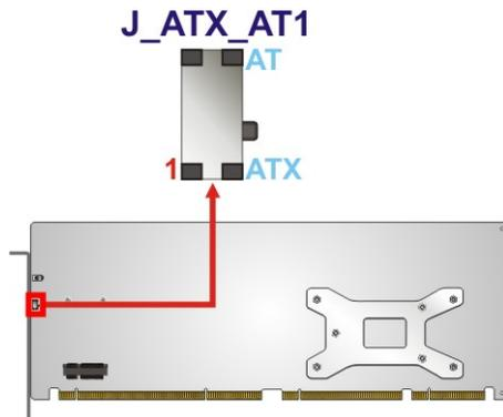
**Figure 4-7: AT/ATX Power Mode Switch Location**
