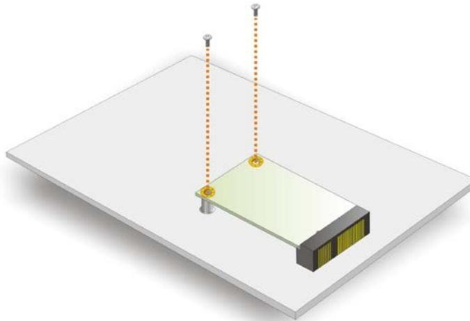
Figure 4-18: Secure the PCIe Mini Card
