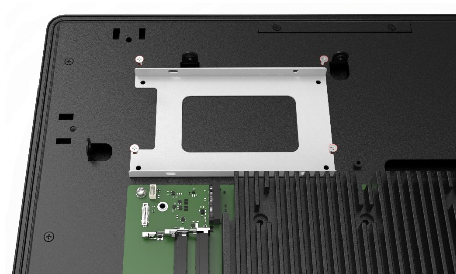
Figure 3-9: Remove the screws from the hard drive bracket
