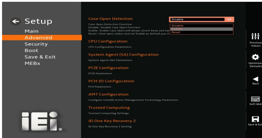
Figure 3-18: Chassis Intrusion Cable Installation (BIOS setting)
