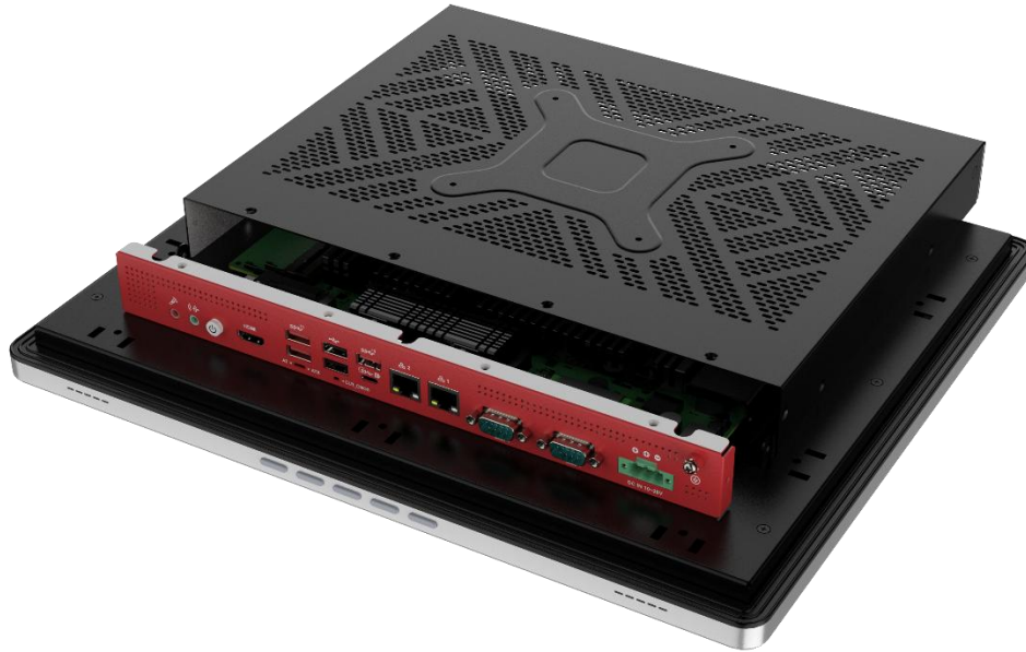
Figure 3-2: Remove the Back Cover
