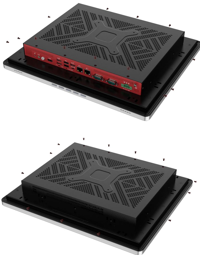
Figure 3-1: AURA-xxx-MTL Series Back Cover Retention Screws
