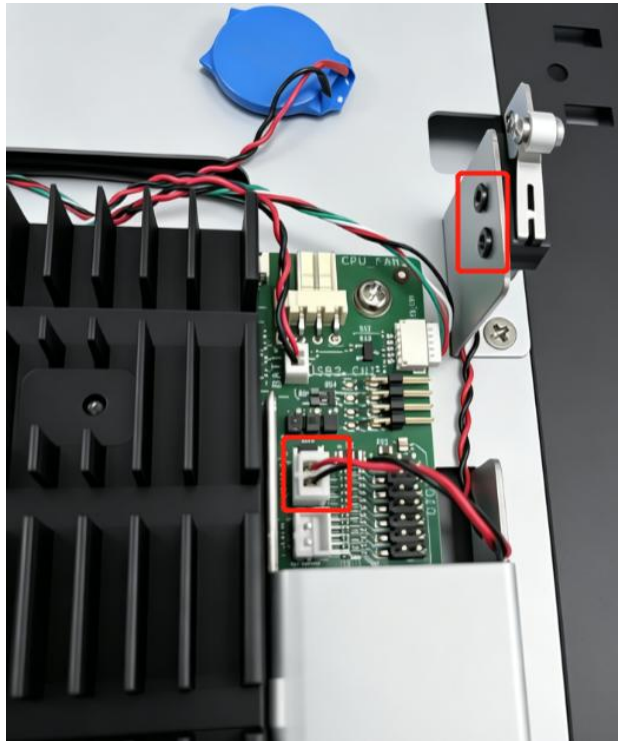
Figure 3-17: Chassis Intrusion Cable Installation
