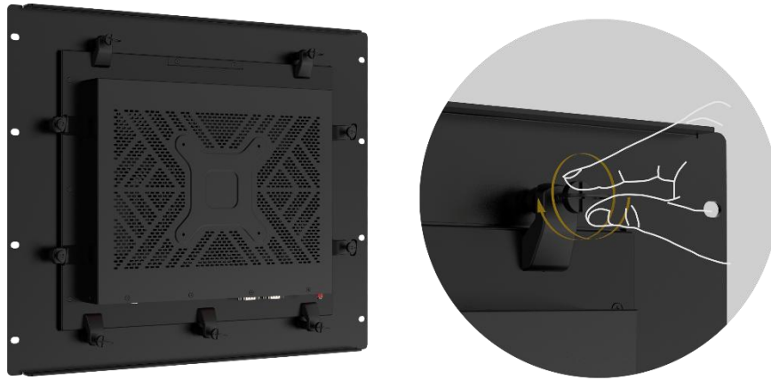
Figure 3-33: Tighten the Mounting Screws
