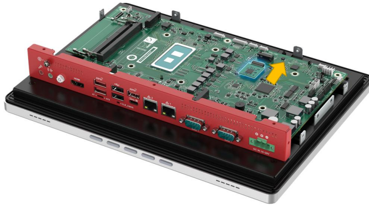
Figure 3-15: Align the TPM module
