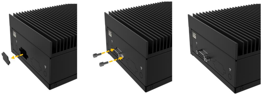
Figure 3-11: Knock Out the Reserved Holes
