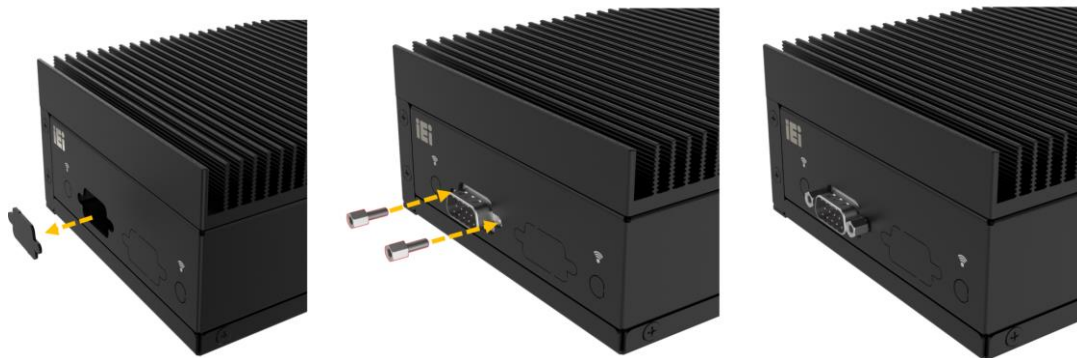
Figure 3-13: Knock Out the Reserved Holes
