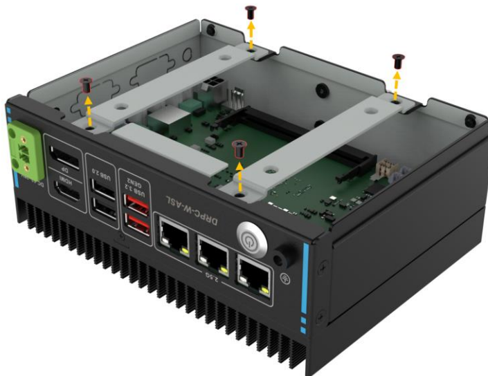
Figure 3-2: Take out the Disk Bracket
