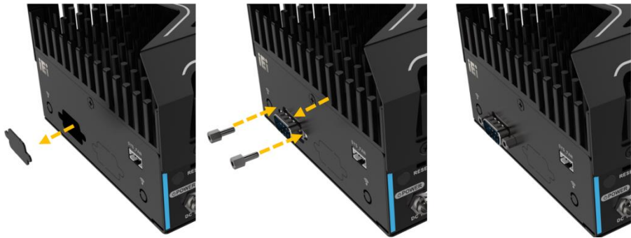
Figure 3-15: Knock out the reserved holes
