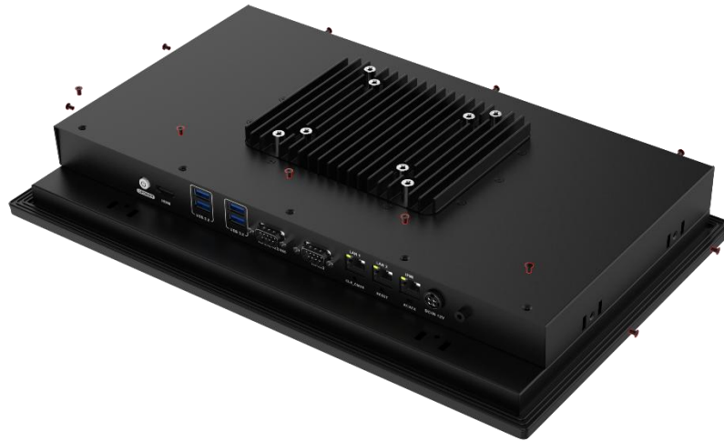
Figure 3-1: Back Cover Retention Screws
