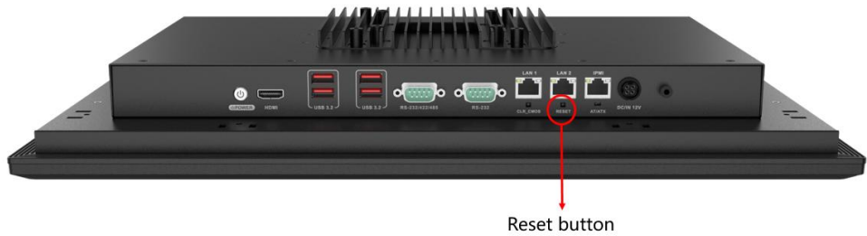
Figure 3-21: Reset Button Location
