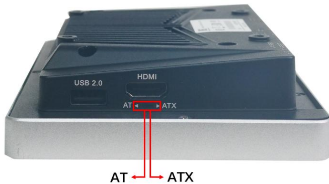
Figure 3-5: AT/ATX Switch Location
