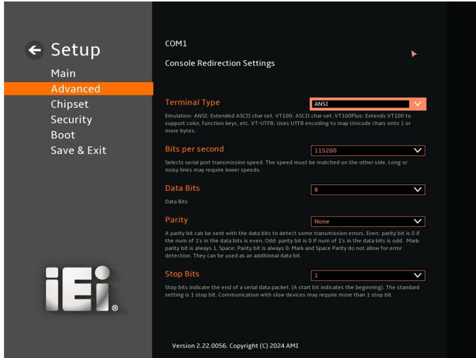
Figure 6-19: Console Redirection Settings
