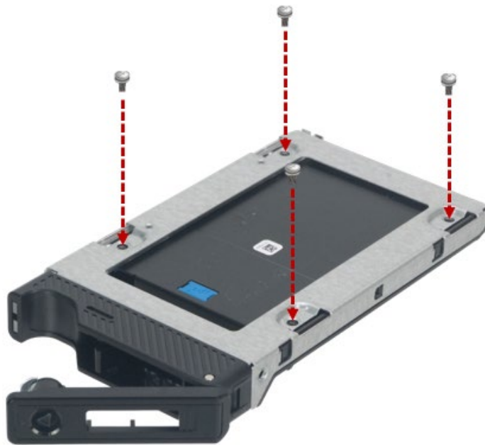
Figure 3-5: Secure SSD to the Bracket
