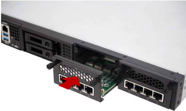
Figure 3-8: Networking Module Installation
