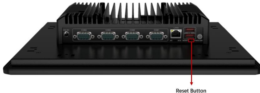
Figure 3-31: Reset Button Location
