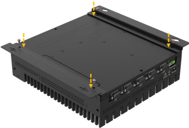
Figure 3-24: Install Wall Mounting Brackets
