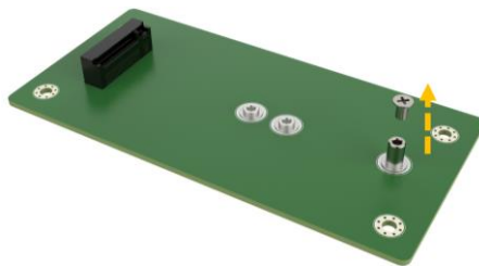
Figure 3-9: Remove the Retention Screw
