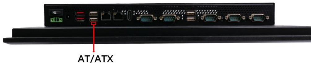
Figure 3-9: AT/ATX Mode Selection
