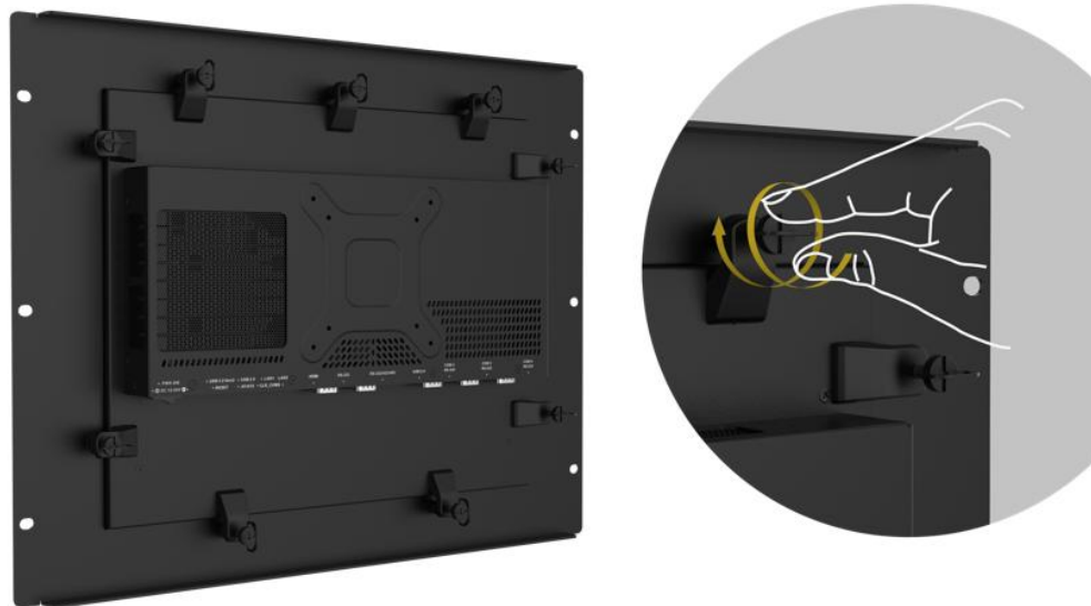
Figure 3-25: Tighten the Mounting Screws
