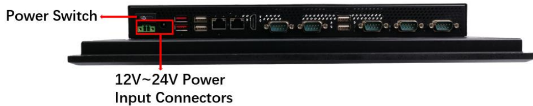
Figure 3-33: Power Connectors and Power Switch
