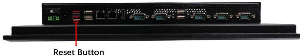
Figure 3-34: Reset Button Location
