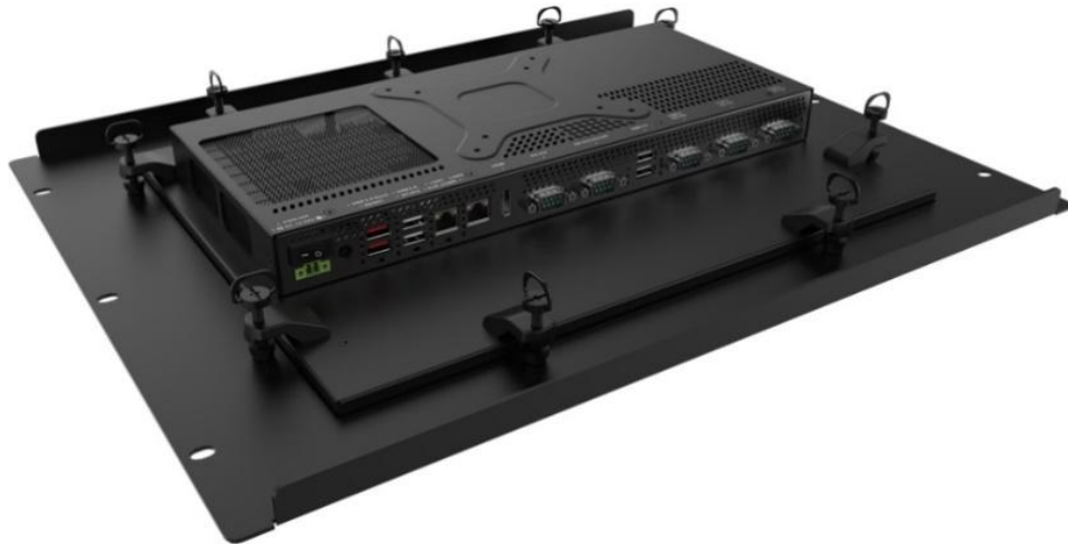
Figure 3-13: PPC2-Cxxx-EHL Series Panel Mount Kit Installation
