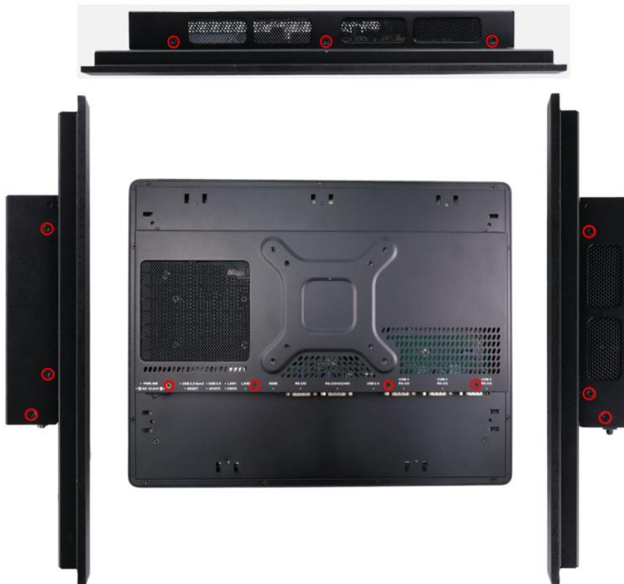
Figure 3-1: PPC2-Cxxx-EHL Back Cover Retention Screws
