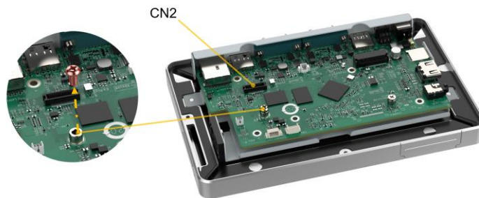
Figure 3-9: WIFI Module Slot Location
