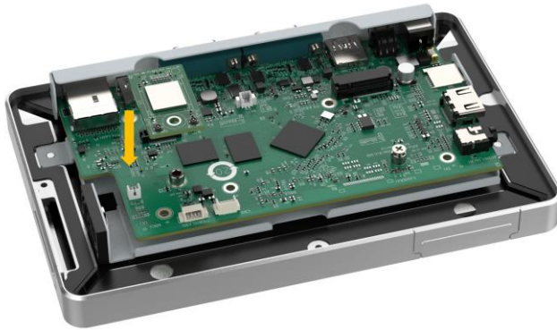
Figure 3-10: WIFI Module Installation
