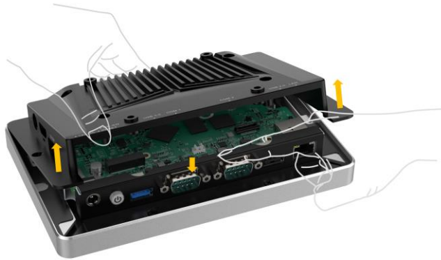
Figure 3-2: Remove the Back Cover
