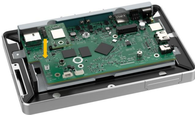
Figure 3-11: Lock Screws and Buckle the Antenna
