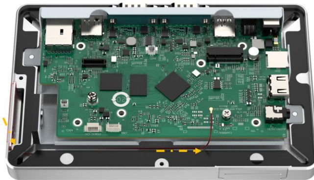
Figure 3-5: Route Antenna to the Module
