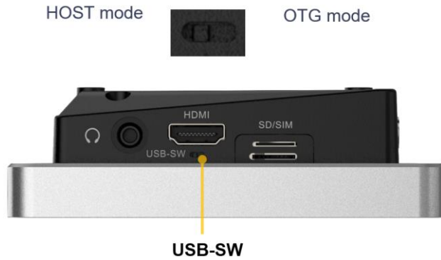
Figure 3-12: USB OTG Switch Location
