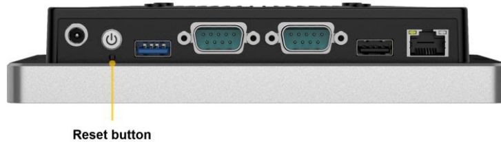
Figure 3-29: Reset Button Location
