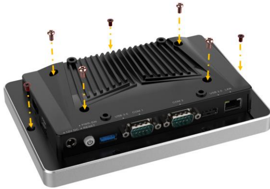
Figure 3-18: Install the Back Cover
