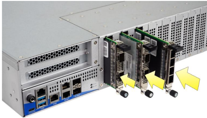
Figure 3-6: OCP 3.0 Card Installation
