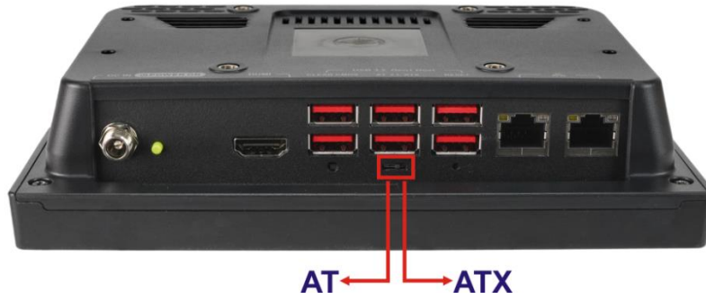
Figure 3-2: AT/ATX Switch Location
