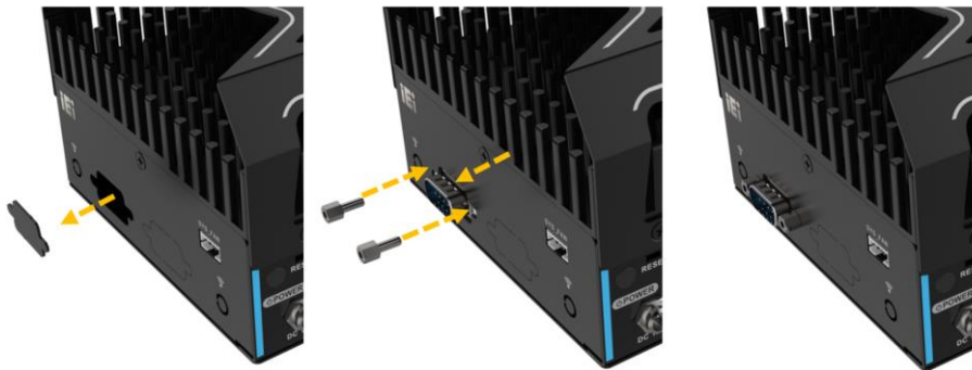
Figure 3-17: Knock out the reserved holes
