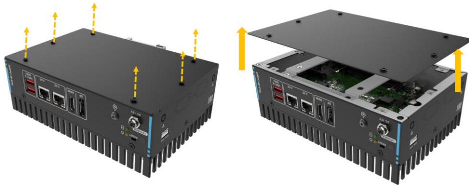
Figure 3-1: Remove the Cover
