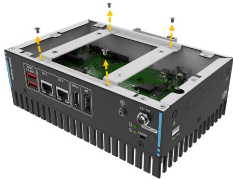
Figure 3-2: Take out the Disk Bracket
