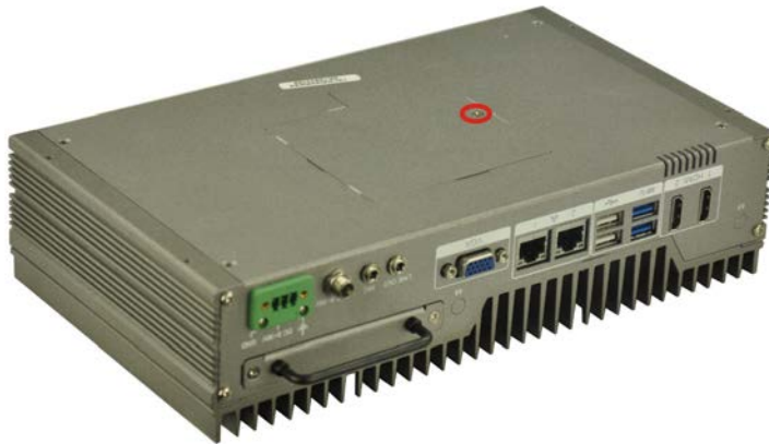
Figure 3-4: Memory Cover Retention Screw
