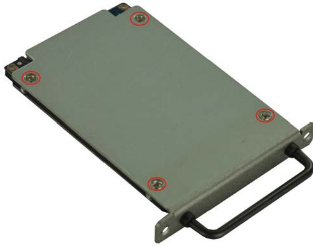
Figure 3-3: HDD Retention Screws
