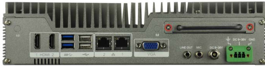
Figure 3-1: HDD Cover Retention Screws
