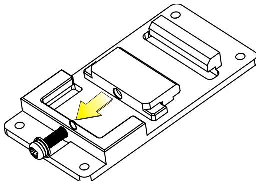
Figure 3-16: DIN Rail Mounting Bracket Preparation
