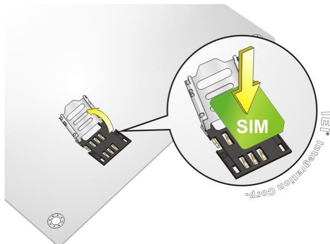
**Figure 3-9: SIM Card Installation**
