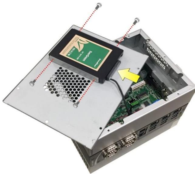
**Figure 3-2: HDD Installation**
