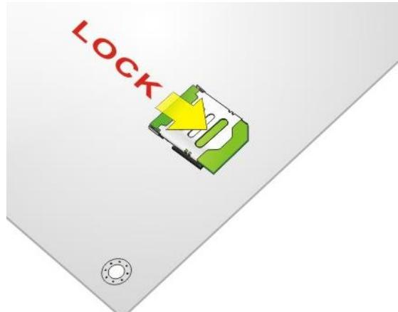
**Figure 3-10: Lock SIM Card Slot Cover**
