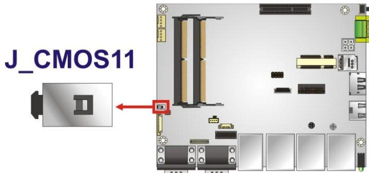
**Figure 4-1: Clear CMOS Button Location**
