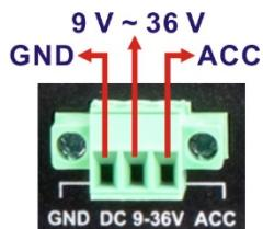
Figure 3-25: Terminal Block Pinouts
