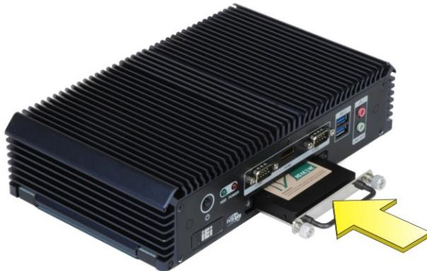
**Figure 3-9: SSD Installation**
