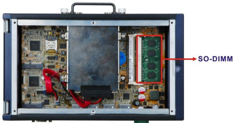
Figure 5-1: SO-DIMM Location
