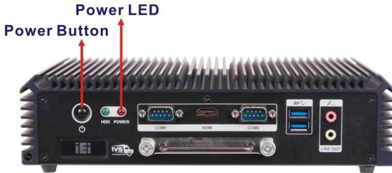
Figure 3-26: Power Button and Power LED
