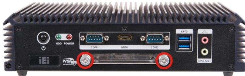
Figure 3-6: SSD Bracket Retention Screws
