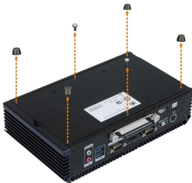
**Figure 3-1: Bottom Cover Retention Screws**
