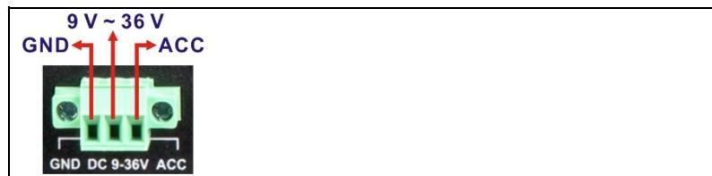
Table 6-14: Power Input Terminal Block (DC\_IN1) Pinouts
