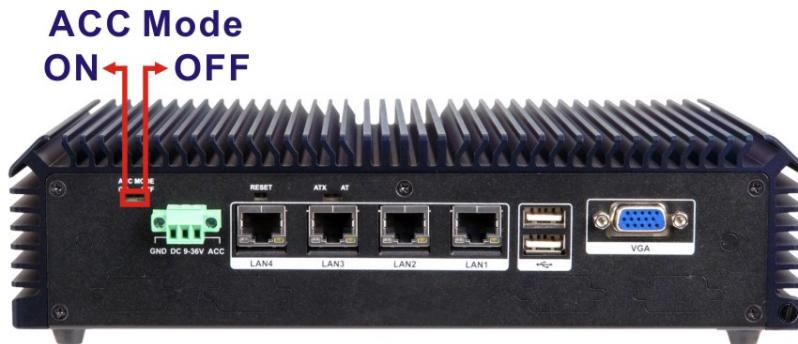
**Figure 3-5:** ACC Mode On/Off Switch Location
