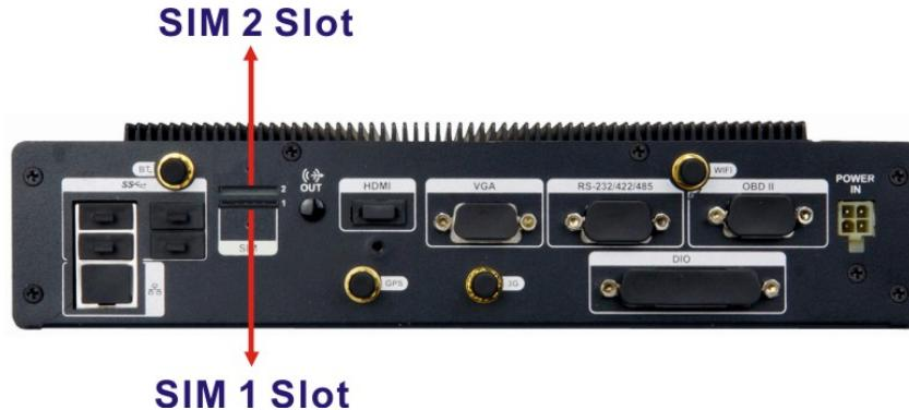
**Figure 3-8: SIM Card Slot Locations**
