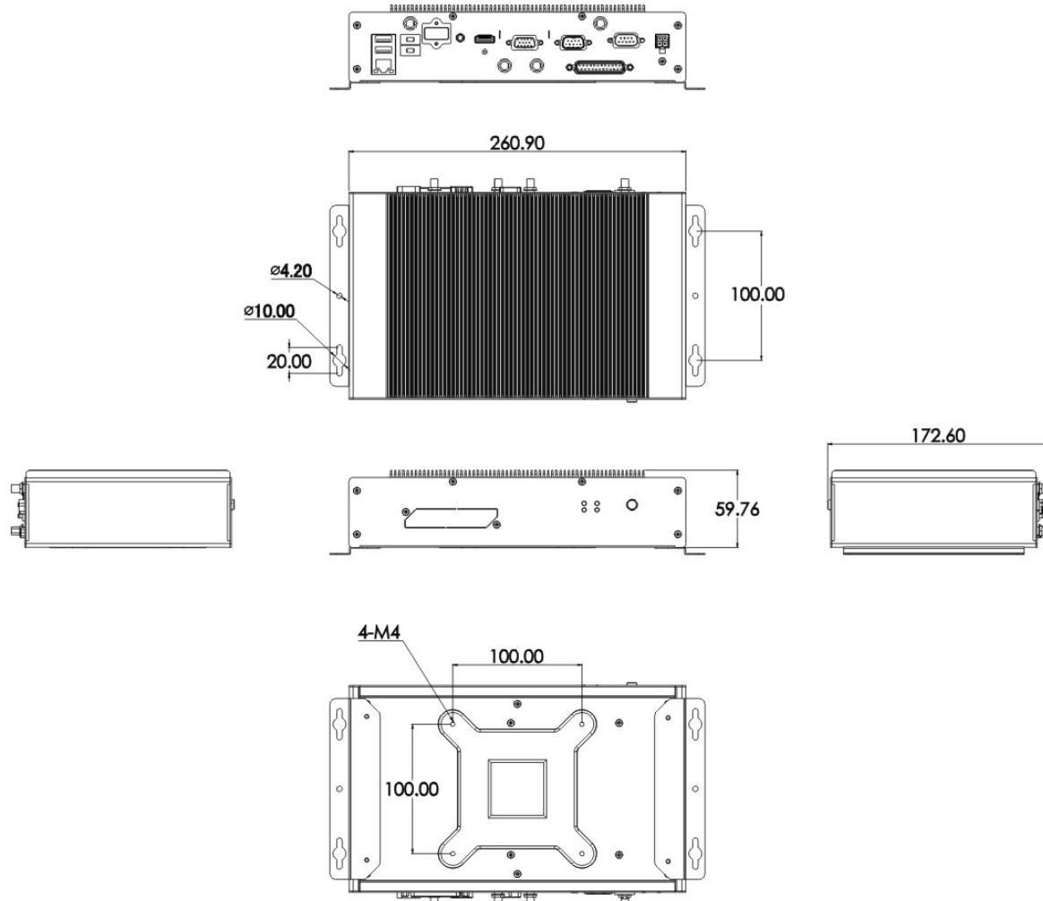
**Figure 1-6: Dimensions (mm)**
