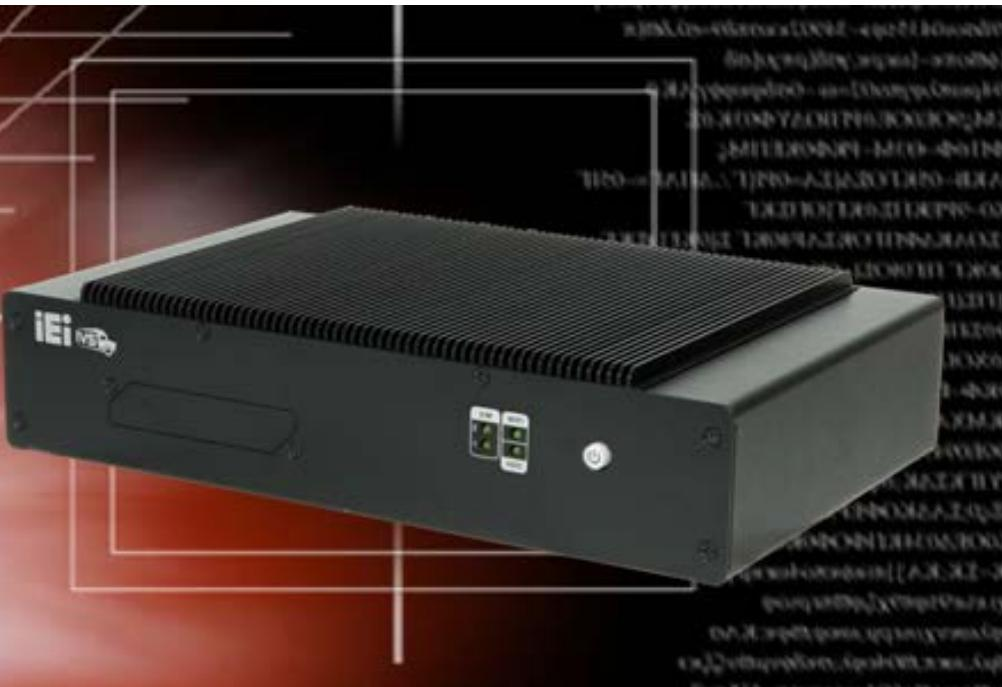
**IEI Fanless Embedded System with Intel® Atom® x7-E3950 Processor, RS-232/422/485, OBD-II, On-board GPS, HDMI, VGA, Dual SIM Slot, RoHS Compliant,**
