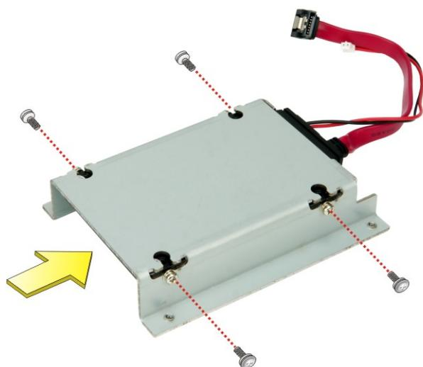
**Figure 3-10: SSD Retention Screws**
