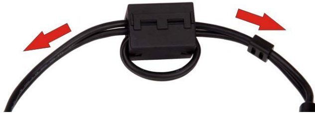
Figure 3-9: Cable Installed with Ferrite Core
