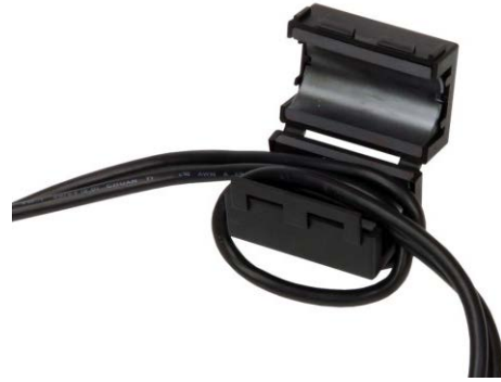
Figure 3-8: Wrapping Cable around the Core
