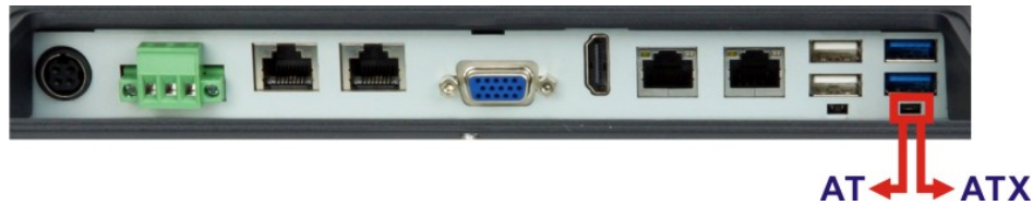
Figure 3-6: AT/ATX Switch Location
