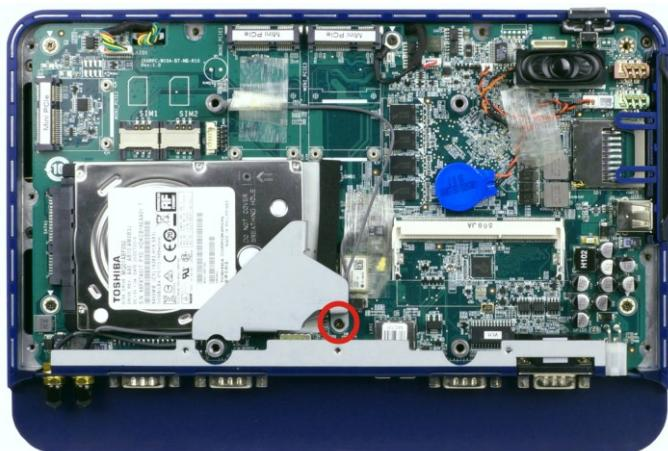
**Figure 3-6: Secure HDD with Holder Bracket**
