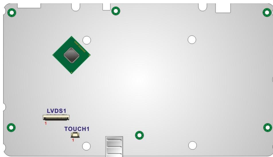
Figure 5-2: Main Board Layout Diagram (Solder Side)
