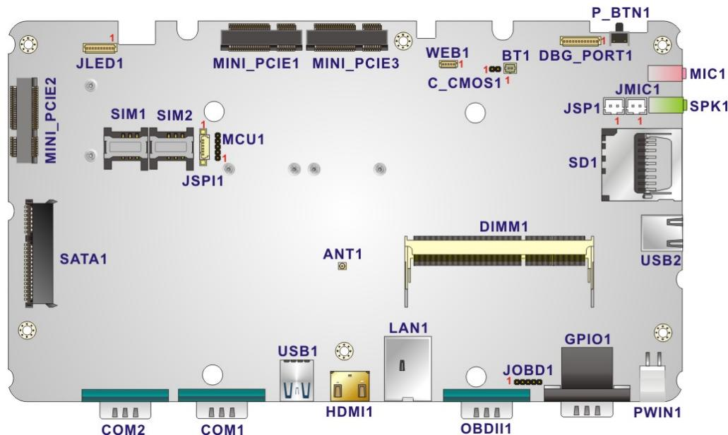
Figure 5-1: Main Board Layout Diagram (Front Side)
