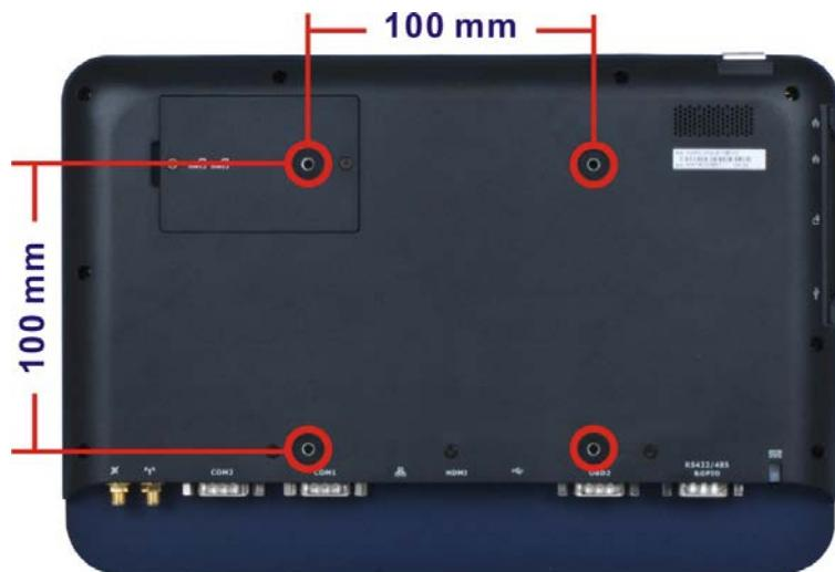
**Figure 3-7: VESA Mount Retention Screw Holes**
