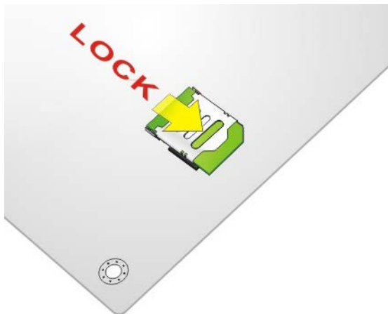
Figure 3-8: Lock SIM Card Slot Cover
