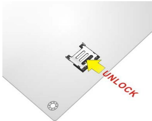
Figure 3-6: Unlock SIM Card Slot Cover
