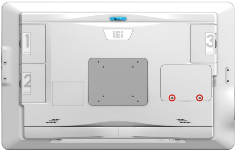
Figure 3-1: HDD Cover Retention Screws
