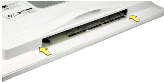
Figure 3-18: Cable Cover Removal
