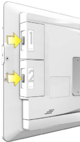
Figure 3-9: Battery Cover Button
