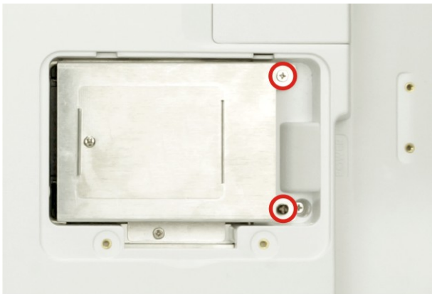
Figure 3-2: HDD Bracket Retention Screws
