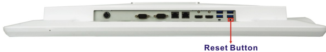
Figure 3-25: Reset Button Location
