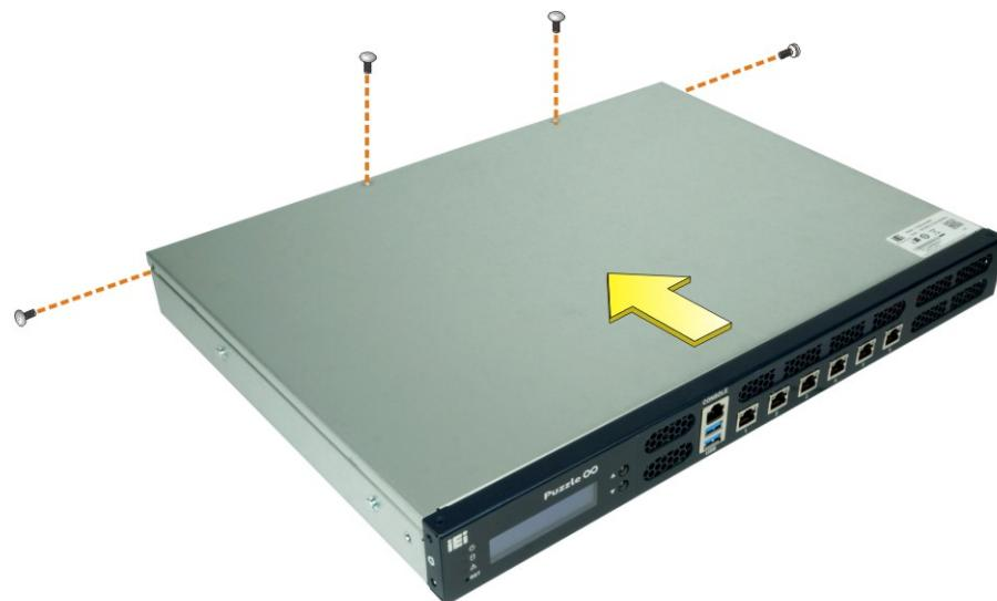
**Figure 3-1: Top Cover Removal**
