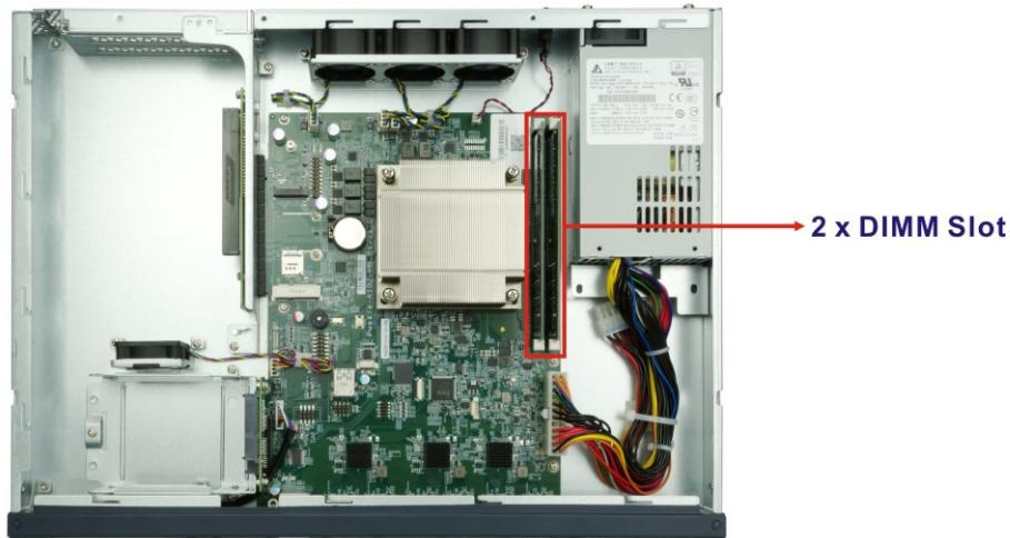
**Figure 3-2: DIMM Slot Locations**
