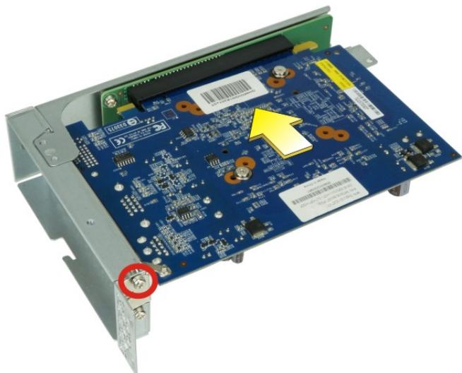
**Figure 3-9: PCIe Expansion Card Installation**
