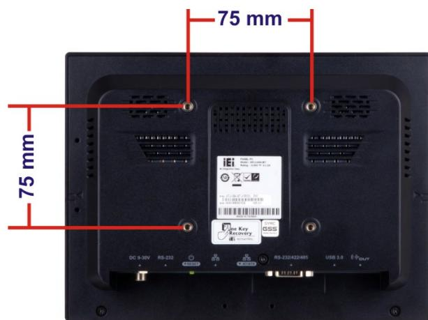
Figure 3-20: Arm Mounting Retention Screw Holes
