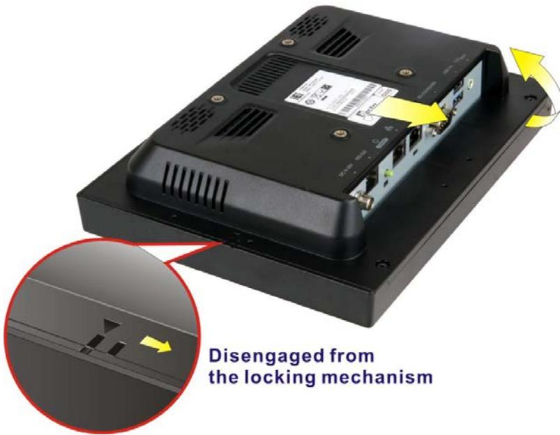
Figure 3-2: Remove the Back Cover
