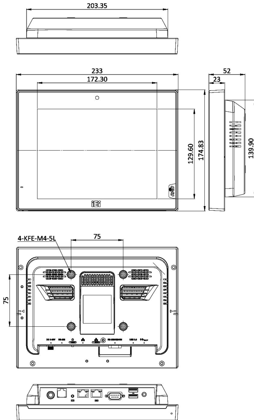
**Figure 1-5: Dimensions (mm)**
