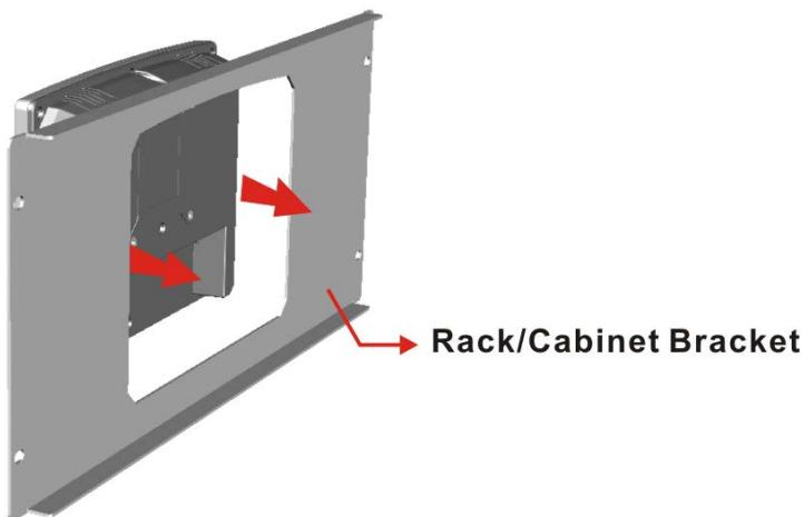
**Figure 3-16: Rack/Cabinet Bracket Installation**
