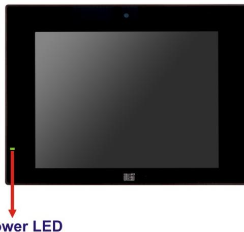
**Power LED****Figure 3-26: Powering On the System**
