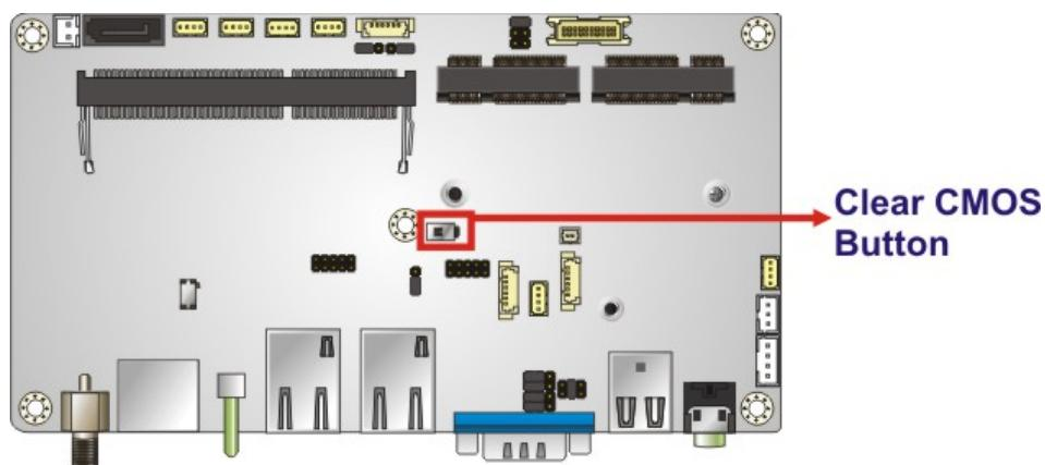
Figure 3-7: Clear CMOS Button Location
