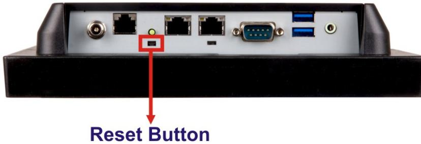
**Reset Button****Figure 3-27: Reset Button Location**
