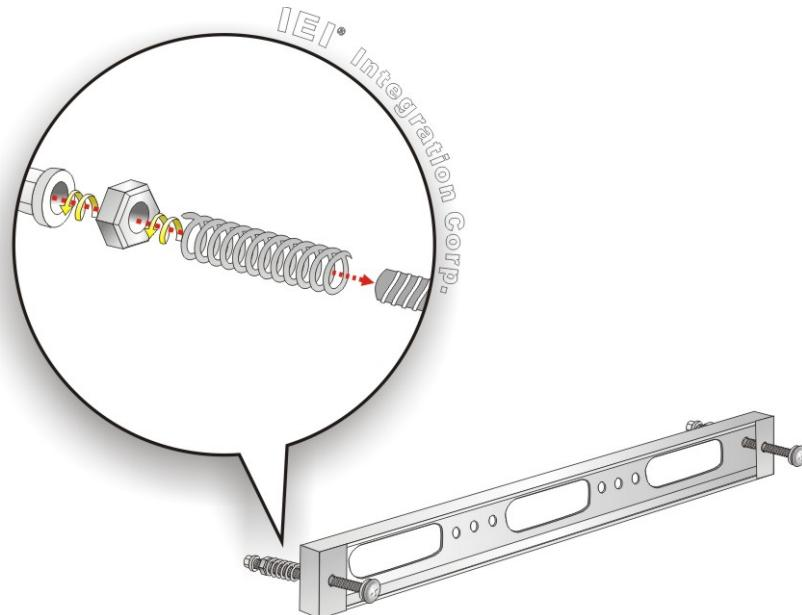
**Figure 3-17: Rack Mounting Kit Installation**
