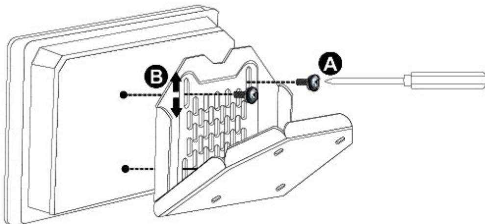
Figure 3-24: Secure V-Stand to System
