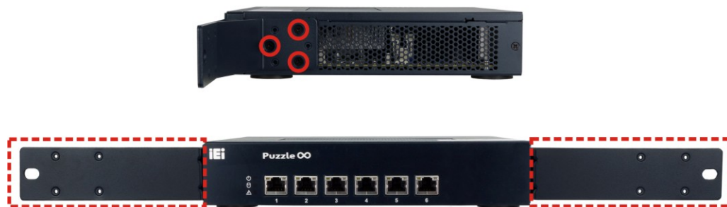
Figure 3-9: Rack Mounting Bracket Installation
