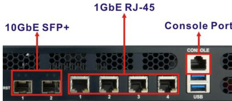
Each Ethernet connector has a physical number (printed on the front panel) and a logical number (under Linux). The following table shows the physical number to logical number relationship on the PUZZLE-M801.
