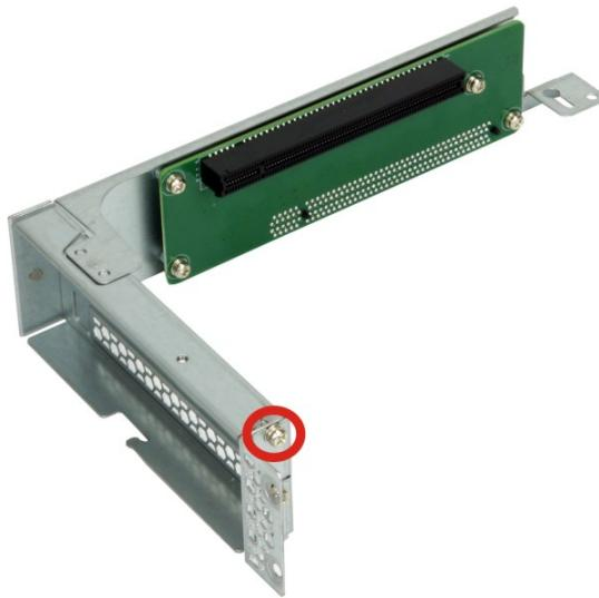
**Figure 3-8: Blank Bracket Screw**
