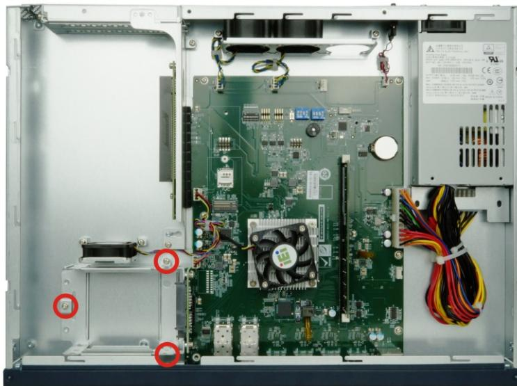
**Figure 3-3: HDD Bracket Retention Screws**
