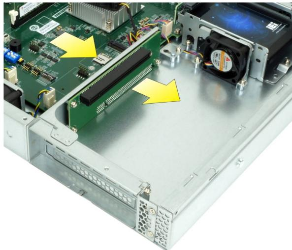
**Figure 3-7: Disconnect the Expansion Slot Module**
