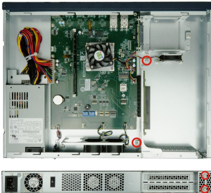
**Figure 3-6: Expansion Slot Module Retention Screws**
