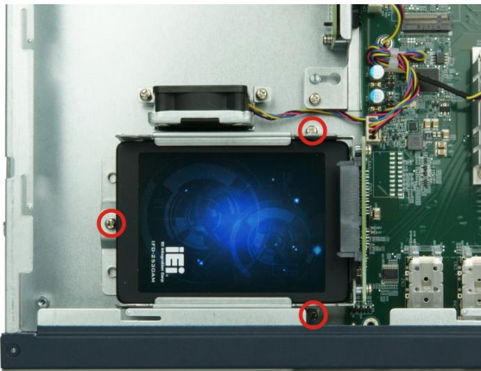
**Figure 3-5: HDD Installation**
