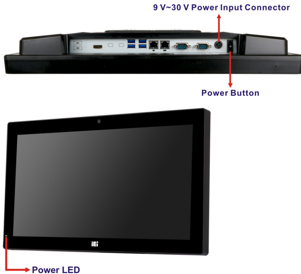
Figure 3-38: Powering On the System
