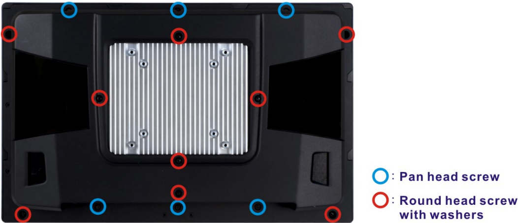
Figure 3-1: AFL3-W15C-ULT3 Back Cover Retention Screws
