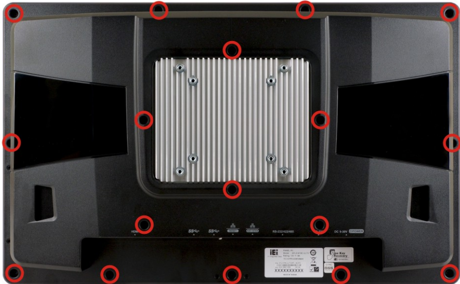
Figure 3-2: AFL3-W19C-ULT3 Back Cover Retention Screws
