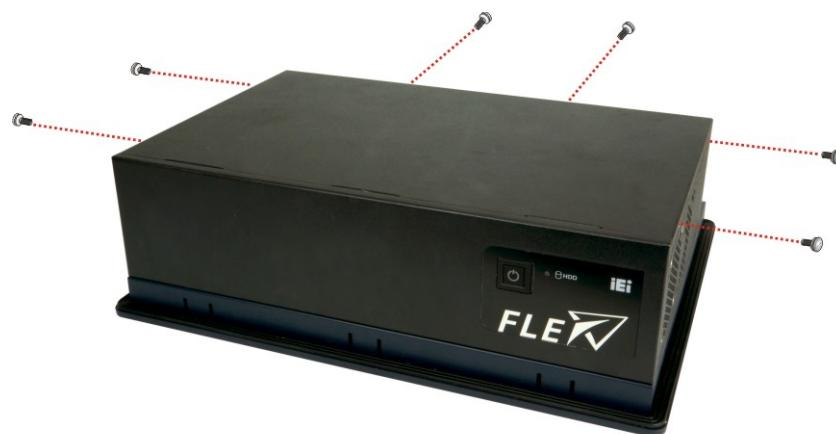
Figure 3-5: Rear Cover Retention Screw Removal
